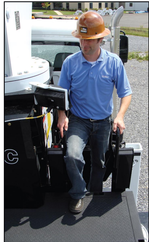
Walk Through Control Stations
